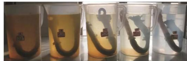
溶液A pH8.80 溶液B pH8.60 溶液C pH7.40 溶液D pH4.40 溶液E pH3.10
